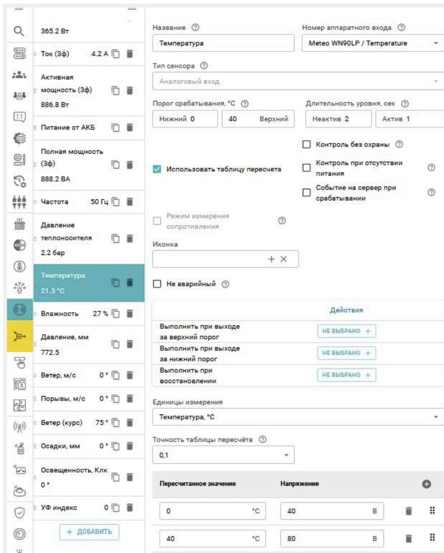
The screenshot shows the configuration interface for a temperature sensor. On the left is a list of sensors, with 'Температура' (Temperature) selected and showing a value of 21.3 °C. The main configuration area includes:
