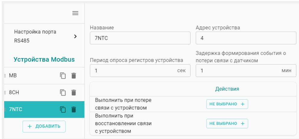
The screenshot shows the 'Настройка порта RS485' (RS485 port configuration) screen. On the left, there is a list of Modbus devices: 'MB', '8CH', and '7NTC'. The '7NTC' device is selected and highlighted in blue. Below the list is a '+ ДОБАВИТЬ' (ADD) button. The main configuration area for the selected device includes:
