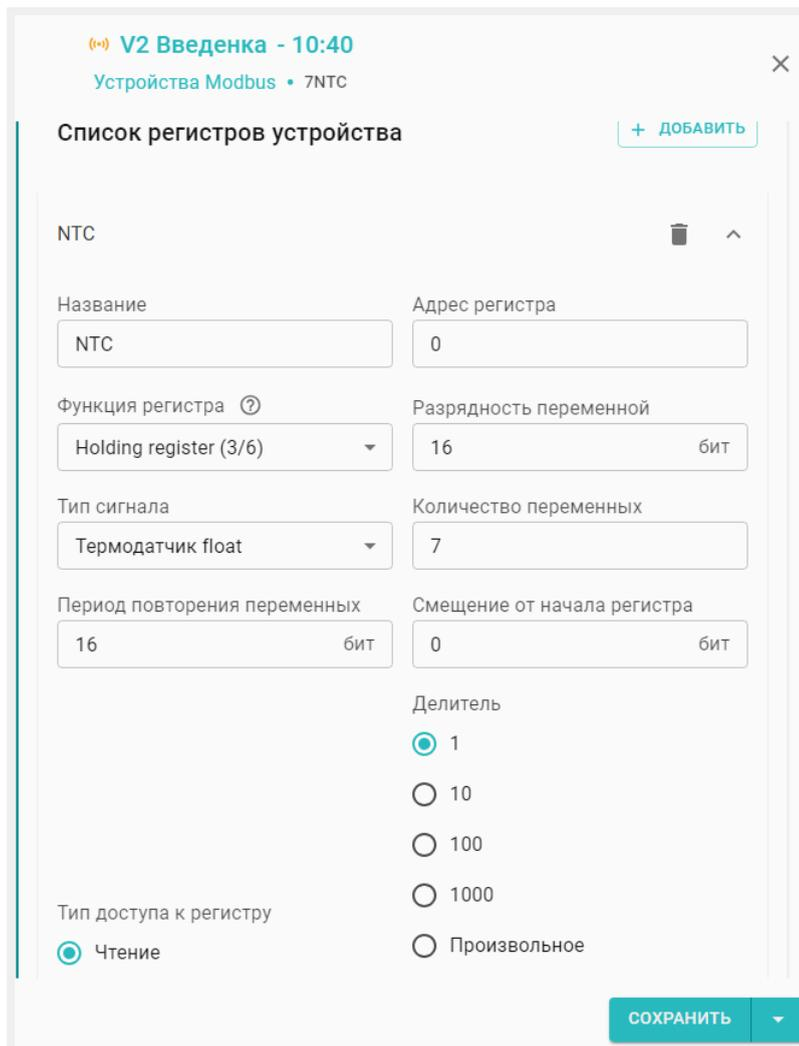
The screenshot shows the 'V2 Введенка - 10:40' (V2 Input - 10:40) dialog box for the '7NTC' device. It is titled 'Список регистров устройства' (Device register list) and has a '+ ДОБАВИТЬ' (ADD) button. The configuration for the 'NTC' register is as follows:
